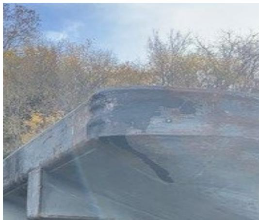
**Figure 7.** Postcasualty photo of the minor damage to the port bow rake of barge *STC 3020*. (Source: Coast Guard)
